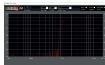
External FIR supports three format of FIR coefficients, namely ".csv", ".txt", ".saf". The first two file formats can be generated by mainstream FIR convolution software and the ".saf" file can be saved and generated from AEQ in the processor. It should be noted that the FIR filter in the input and output part of the DLM series works at a sampling rate of 48kHz and a maximum of 512 taps.
