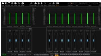
A new function called "keep linked CHs level offset" has been added. The conventional linkage channel will link the level faders together. For some active speakers the output level ratio should remain the same. When this happens select "keep linked CHs level offset".
