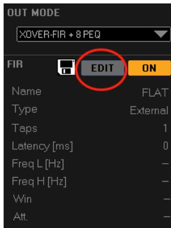
Provides three guides of high-pass / low-pass / band-pass, you can enter the frequency that needs to be band-passed according to your needs, choose more or less taps, slopes from -20dB to -120dB/oct, and multiple window function types. Click save at the red circle (here we use band pass filter as an example).
