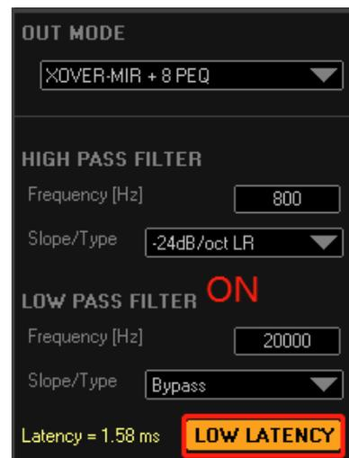
For the FIR filter two modes can be selected, FIR+8 segment PEQ, FIR+IIR high and low pass with a slope of up to -24dB + 4 segment PEQ.
