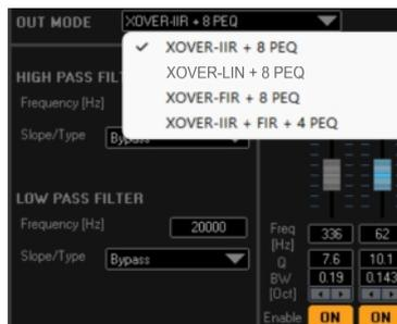
In the high and low pass filters of IIR we provide three types of traditional Butterworth / Linkwitz-Riley / Bessel slopes ranging from -6dB/oct to -48dB/oct.
