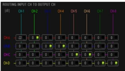
In the input matrix you can arbitrarily route the signal from the input processing channel to the output processing channel. The default sending volume is 0dB which is equivalent to group output. When choosing different sending volume it is equivalent to real Mixing Matrix sending.
