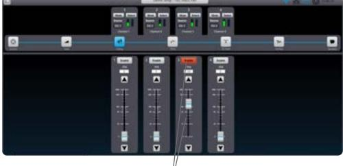
**Delay:** opens a window where you can set the delay in ms of the four channels, regardless of what channel is selected. Values can be set with the fader, keyboard arrows or by dialling in the desired level.
