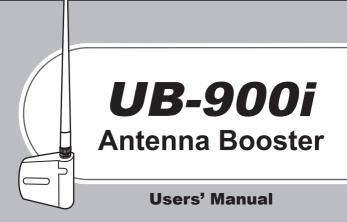
UB-900i is designed to compensate signal loss on long antenna cables or passive antenna splitter. One UB-900i can compensate 10dB of cable attenuation which is about 20 meters of RG-58 cable. This product is powered by power output from antenna distributor UA-960 or from receivers' BNC connecter. DC power supply is indicated by a red LED.
