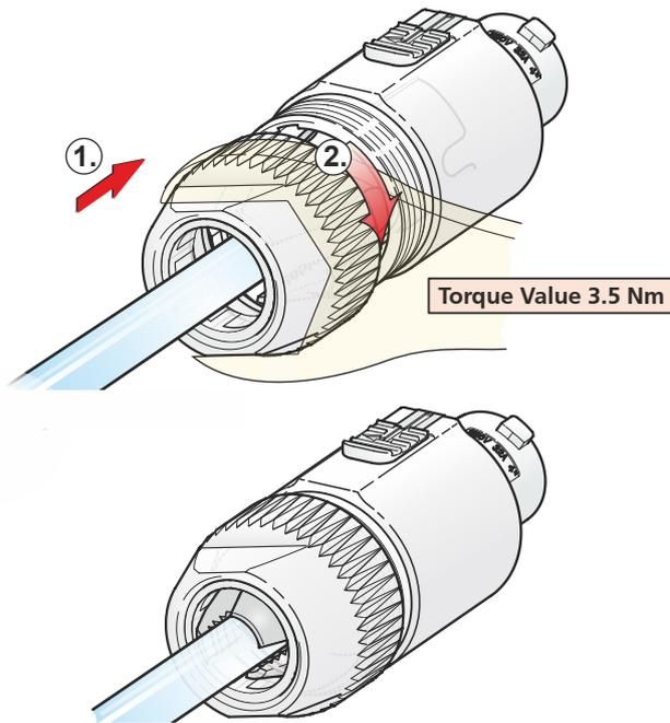
D 1. Push insert and chuck into housing.
